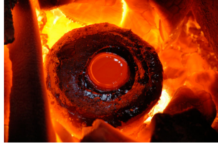
FIGURE 8 The silver without the “veil” of oxides, at the end of the cupellation process. © Nicolas Thomas.
