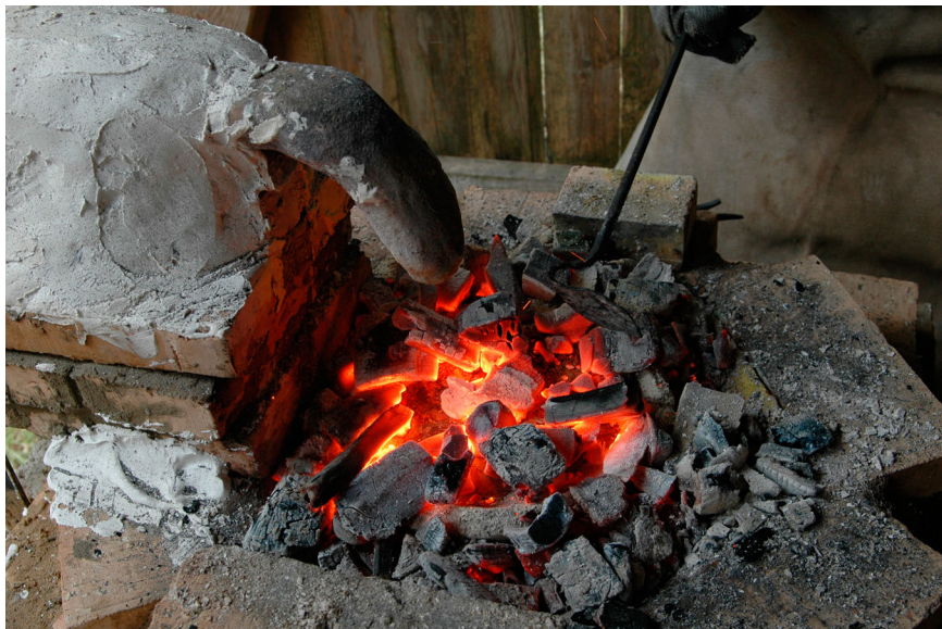
FIGURE 5 Cupellation process, with bellows blowing on the ash-filled crucible from above (the crucible is under the charcoal). © Nicolas Thomas.
