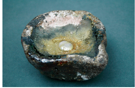
FIGURE 9 Silver button, still covered with litharge and oxides after a cupellation. © Nicolas Thomas.
