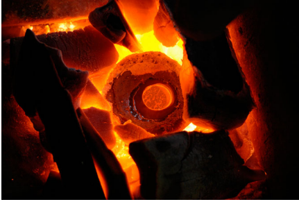
FIGURE 7 Molten silver with a “veil” of oxides during the cupellation process. © Nicolas Thomas.
