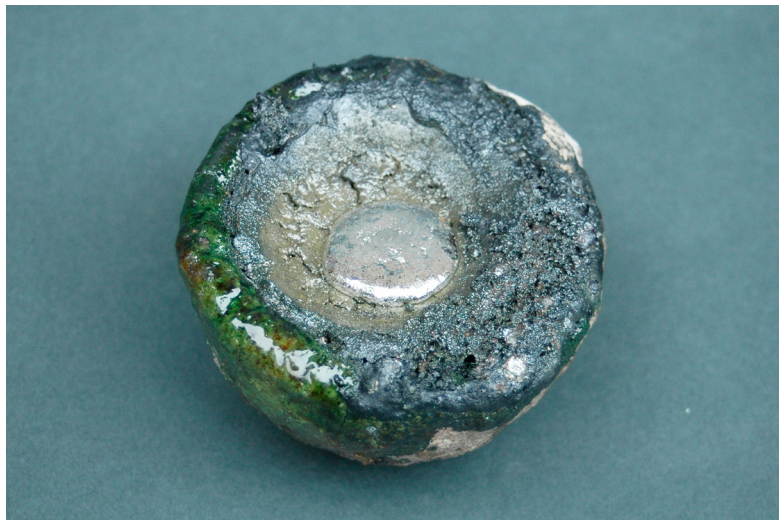
FIGURE 3 The silver button at the bottom of an ash-filled crucible after the cupellation process. © Nicolas Thomas.
